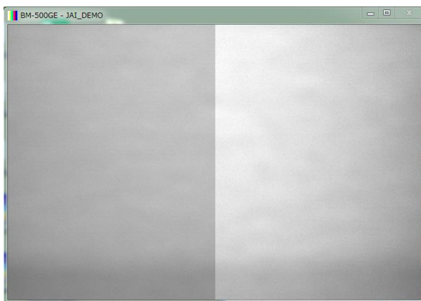
Fig. 1: Unbalanced tap example
