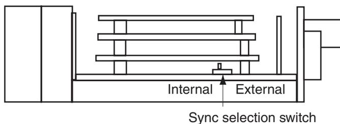
FIGURE 5. Mode Selection Switch (DIP Switch)
