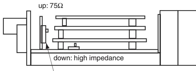
Up position is 75 Ω for HD and VD inputs.
