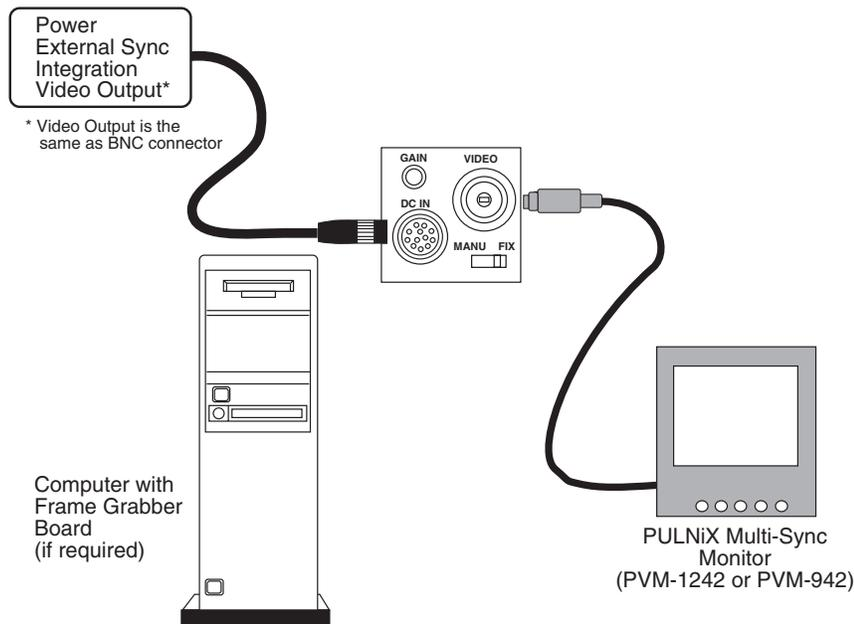
**NOTE:** Additional cable interface may be required from the frame grabber board manufacturer.
