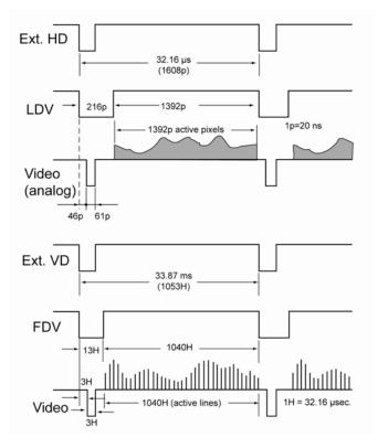
It is important to meet the exact starting pixel at LDV and the starting line of FDV. If the starting pixel or line is shifted due to the image capture configuration, then the interpolation software can be adjusted for the correct starting point. In figure A, if the first pixel is shifted (missed), the color interpolation should start with G-R. If the first line is missed in A, the interpolation order will be B-G.
