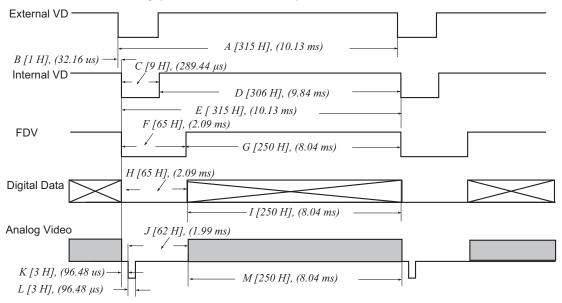
4. Async Shutter Reset Timing (Partial Scan 250 Lines)
