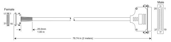
The TM-1402 camera uses the cable 30DG-02 from JAI, Inc. as a digital output cable. This cable has a 31-pin AirBorn connector on the camera end and a 37-pin D-sub male connector on the other end. Contact your JAI, Inc. representative regarding availability of interface cables for specific frame grabber models. Pinout configuration for the digital cable is shown below.
