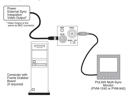
*NOTE:* Additional cable interface may be required from the frame grabber board manufacturer.
