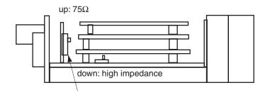
Up position is 75  $\Omega$  for HD and VD inputs.
