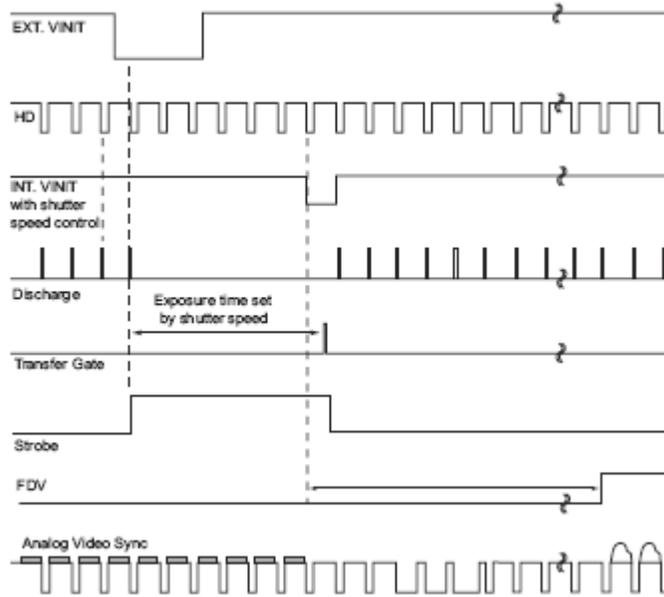
The camera operates the reset and shutter in the same way as the external pulse width control mode. When the external VINIT pulse is applied, internal VINIT is latched to HD and the internal VINIT is delayed to set up the shutter speed period. The shutter speed is controlled by communication software from “1” to “8.” Video output timing starts right after the internal VINIT and single shots. FDV is output at the internal VINIT timing.
