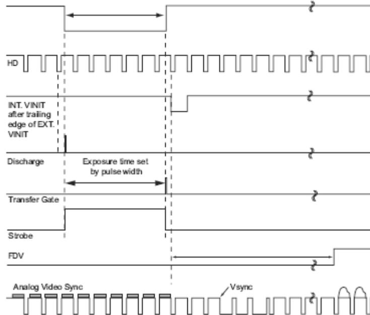
The RM-6740CL camera also has read-out-inhibit control (ROI) to control the vertical clock start (Async Shutter #9). When ROI is low, V-clock is stopped and the transferred charges remain in the vertical shift registers, which work like CCD memory. When the ROI is high, it clocks out the CCD data. This helps a single frame grabber process multiple images in pipeline processing (sequential process).
