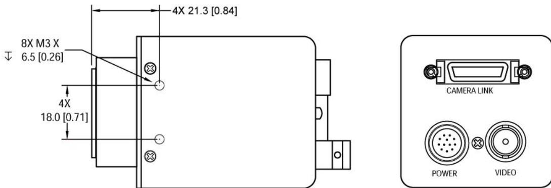
*Caution: When mounting the camera to any fixture, do not use screws that extend more than 5 mm into the camera housing to avoid possible damage to the internal circuitry. For attaching the tripod mounting plate, only the supplied screws should be used.*
