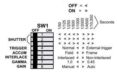
The shutter values are given for a CCIR camera having the factory settings. Shutter values for other setups and EIA cameras can be seen in table 7.1.3.
