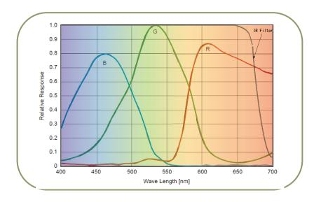
Fig. 36. Spectral response for CB-030GE/CB-030GE-RA
