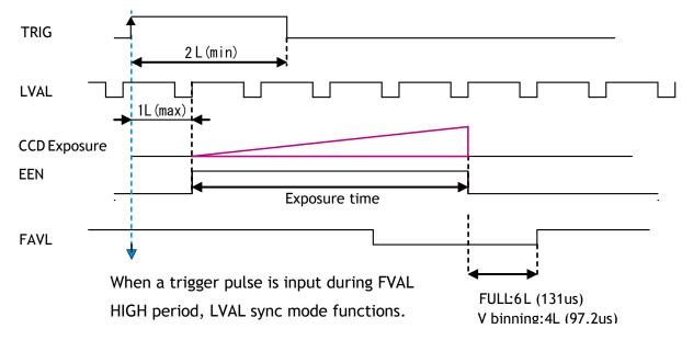
Fig. 28 Edge Pre-select LVAL sync Timing
