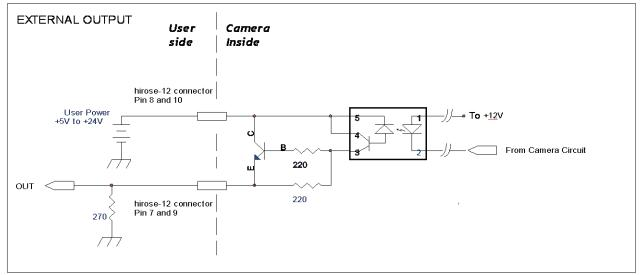
Fig.11. External Output Circuit, OPT OUT 1 and 2
