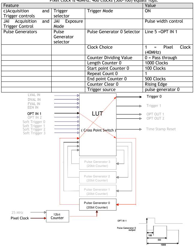
Fig.13. Pulse Generator Timing Example 1
