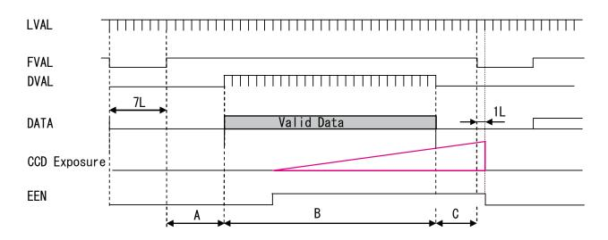
Values for vertical timing in partial scan continuous mode.
