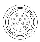
Fig. 4. 12-pin connector.
