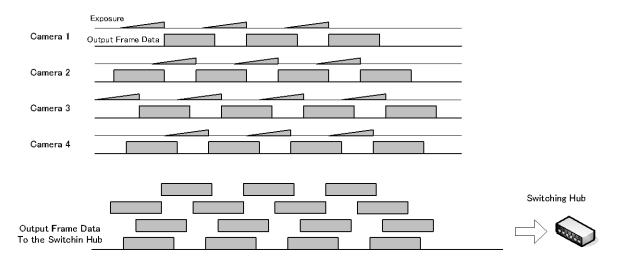
• The packet delay should be set larger. The data traffic is controlled by the buffer of the hub. It is necessary to check the buffer value of the unit.
