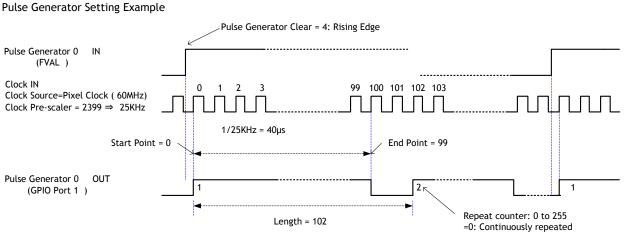
Fig 8. Pulse generator setting example
