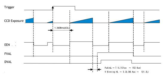
Note: When PE is set at 511 or the shutter is set at OFF, EEN is always HIGH.
