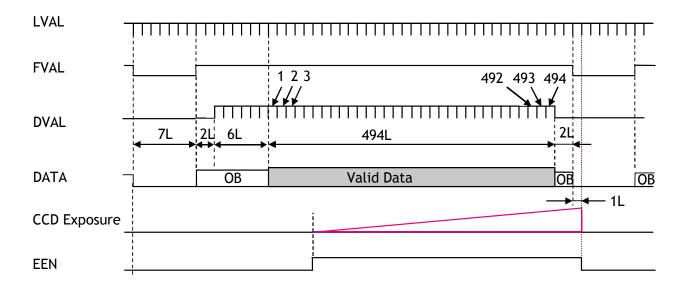
Fig. 20. Vertical timing for full scan
