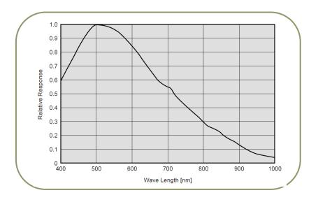
Fig. 35. Spectral response for CM-030GE/CM-030GE-RA
