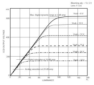
The typical interline transfer CCD has fixed noise levels based on dark current (thermal or KT noise), pattern noise, and the operating clock speed. In general, the level of the 40 MHz pixel clock CCD at room temperature is around 20 to 30 electrons. The maximum capacity of CCD charges is limited by the well capacity at saturation. The range is limited by the structure and the pixel size.
