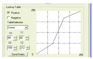
Enter  $X_1$ ,  $Y_1$ ,  $X_2$ ,  $Y_2$  values directly to adjust the knee curve. In the integrated camera software, the look-up table can also be controlled interactively. The Table Selection pull-down menu allows you to select the Linear or Gamma 45 option. This control also allows you to check the positive or negative box to choose an image option.
