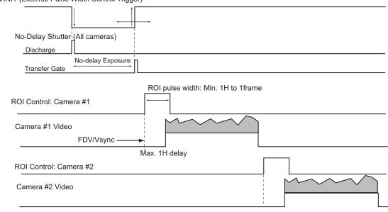
VINIT (External Pulse Width Control Trigger)
