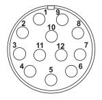
Pin #1 is Ground and pin #2 is +12V DC. Table 6 shows the pin-out table.
