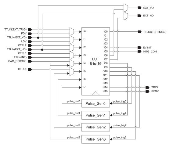
Inputs I0 through I7 can be either external or internal inputs to the look-up table. The outputs are used by the imager part of the GE camera.
