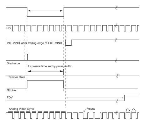
The TM-4100GE camera also has read-out-inhibit control (ROI) to control the vertical clock start (Async Shutter #9). When ROI is low, V-clock is stopped and the transferred charges remain in the vertical shift registers, which work like CCD memory. When the ROI is high, it clocks out the CCD data. This helps a single frame grabber process multiple images in pipeline processing (sequential process).
