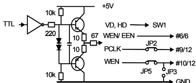
Fig. 7. HD, VD, PCLK, WEN and EEN output.
